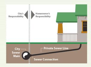
Waste travels from your home's plumbing system through the lateral to the municipal sewer main. Waste then travels through the municipal sewer mains to a wastewater treatment facility where the waste is properly managed.
